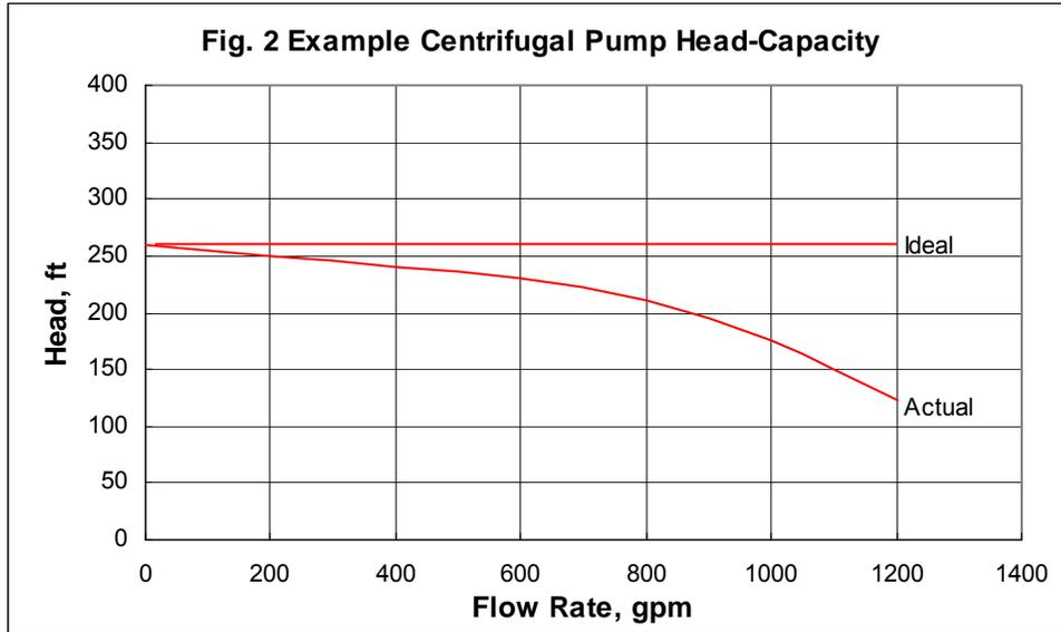
Centrifugal pump generates a head (in height of fluid column) which is independent of fluid density. When the density of the pumping fluid is changed, the pump head is constant at the constant pumping rate, yet the **differential pressure** is changed according to the fluid density.
