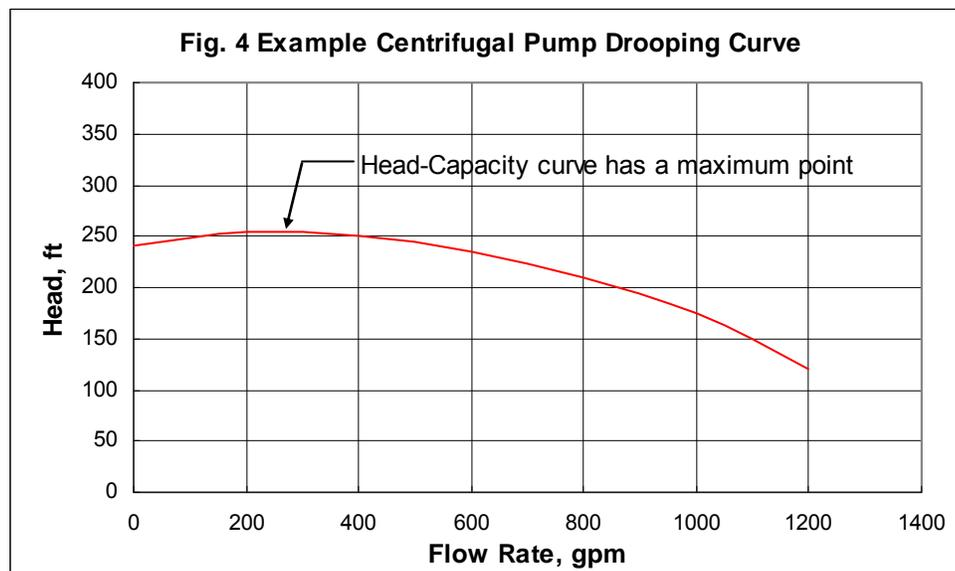
In addition to the head-capacity relationship for the hydraulics, each set of centrifugal pump performance curve typically also shows pump mechanical efficiency, the required net positive suction head, and the brake horsepower vs. capacity. Accompany parameters for the pump are impeller size and speed.
